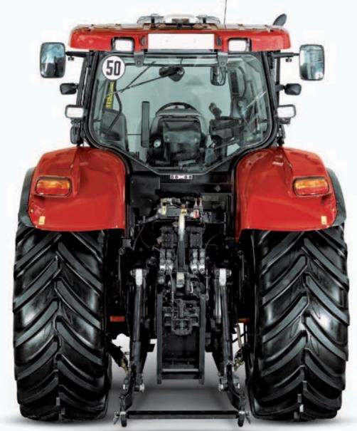
**Fender-mounted controls** for hitch, one remote and PTO make it safe and easy to hitch up implements single-handed.
